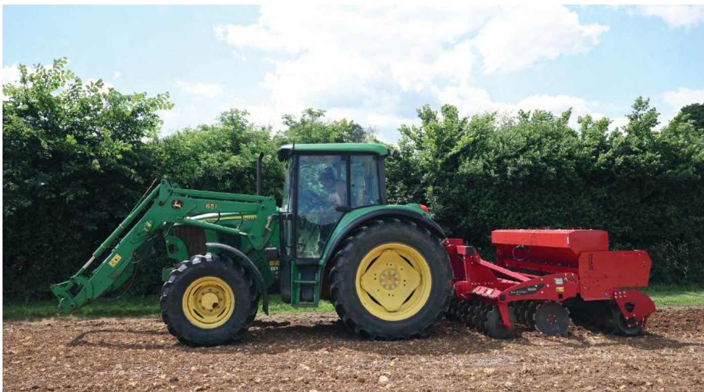
MEADOW CREATION: 3m roller feed seed box mounted on 3m discs surface sowing a meadow mixture at 2\text{g/m}^2 onto the surface of prepared bare soil
