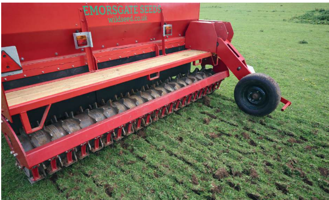
MEADOW RESTORATION: 3m roller feed seed box mounted on 3m discs surface sowing a meadow mixture at 2\text{g/m}^2 onto the surface of scarified species poor grassland
