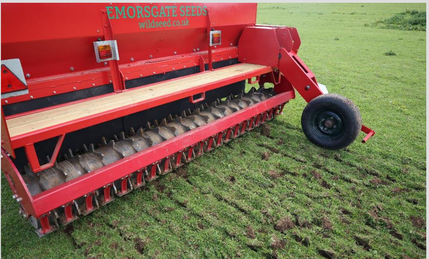
MEADOW RESTORATION: 3m roller feed seed box mounted on 3m discs surface sowing a meadow mixture at 2\text{g}/\text{m}^2 onto the surface of scarified species poor grassland
